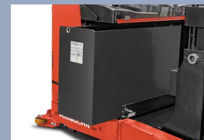
Battery side roll out
